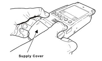
2. Drop the supply into the well. Make sure the supply unwinds from the top as shown.
